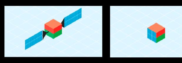
Mounted solar panels: Cover the surface of satellite, collecting sunlight to provide power.
