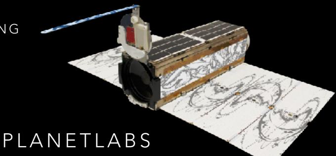
DISASTER MONITORING **CUBE** SAT DIMENSIONS: 10 X 10 X 34 CM (MINI) MASS: 5 KG ORBIT: LOW-EARTH ORBIT INSTRUMENTS: 4
