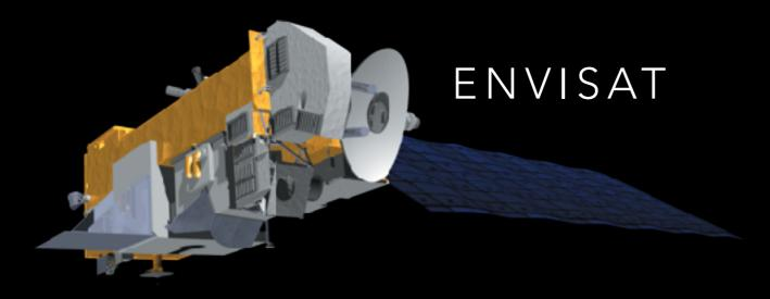
ATMOSPHERE AND OCEAN MONITORING DIMENSIONS: 2.5 × 2.5 × 10 M (LARGE) MASS: 8,211 KG ORBIT: LOW-EARTH ORBIT INSTRUMENTS: 9
